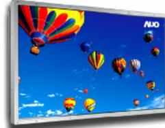
This TFT-LCD (Thin Film Transistor Liquid Crystal Display) Module has a TFT active matrix type liquid crystal panel 1366 x 768 pixels, and diagonal size of 42 inch. Each pixel is divided into Red, Green and Blue sub-pixels or dots which are arranged in vertical stripes. This TFT-LCD has been designed to apply the 8-bit 1 channel LVDs interface method. It is intended to support displays where high brightness, wide viewing angel, high color saturation, and high color depth are very important.
