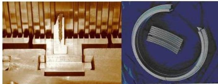
Figure 13: Inter-stage Packing Brush Seal
